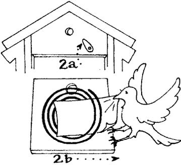
2. Place the clock face down. Open the back of the clock by turning the small metal latch (2a). Remove the back panel and pull the paper out from behind the spiral gong wire on the inside of the back panel (2b).
