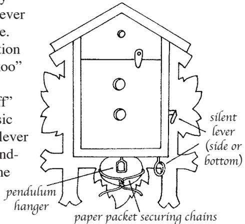
2. **Start the clock and place it “in beat.”** Gently swing the pendulum to one side to start its momentum and initiate the clock’s ticking. Listen carefully- if the ticking lacks a perfect or regular rhythm, your clock will run for only a few minutes and then stop. Swing the base of the clock a little to the left or right until the ticking is even. Many owners place a faint pencil mark on the wall along one side of the clock. This can be used to reposition the clock if it is accidentally moved.
