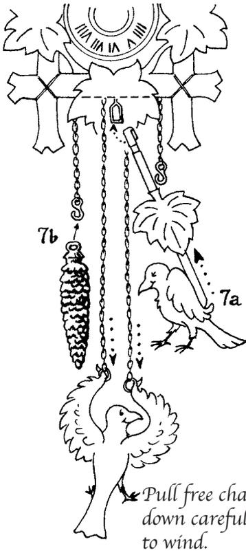
7. Attach the pendulum to the “U” shaped wire pendulum leader at the bottom of the clock (7a). Then attach the weights to the hook ends of the chains (7b).
