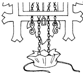
6. For maximum running time, hang your clock approximately 6' off the floor on a secure, strong nail or hook. At this height, the round chain ends should hang about 6" off the floor. Running time will be a full day or week depending on the clock mechanism.
